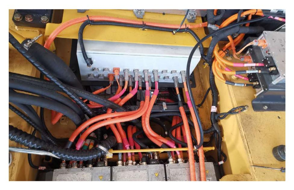
→ Tailored PDU with HV wiring and VECTOPOWER inverters
