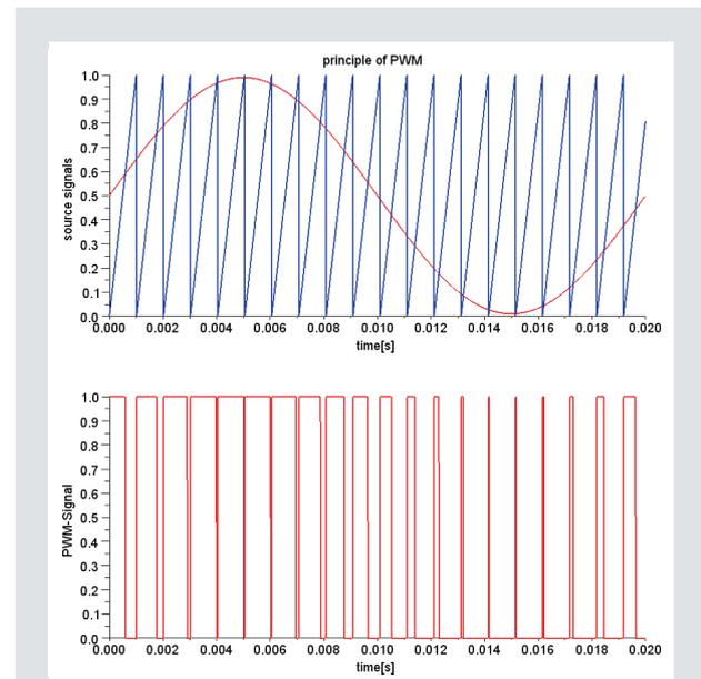
A timer for a sawtooth cycle is shown in blue. The clocked voltage curve in red (lower figure) then yields the smoothed red curve (upper figure) with a roughly sinusoidal voltage curve as an average value.
