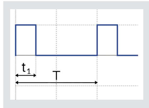
**Application:** Applying such a PWM method to all three phases produces a 3-phase rotating field with an almost sinusoidal curve of the average voltage at the motor terminals. This is referred to as sine commutation.
