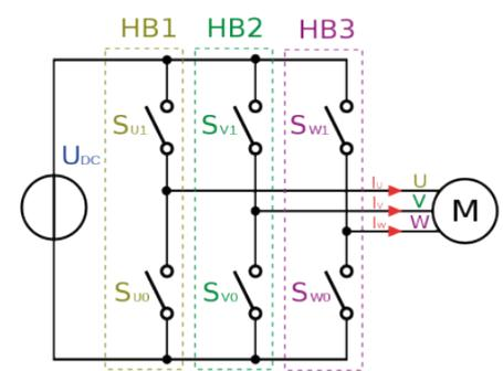
ones. The most common three-phase rotating fields are inverters with six „switches“ (here usually IGBT).
