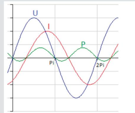
The example shows a relatively „poor“ cos phi in the range of 0.7. It can be seen that the apparent power P can also take on negative values.
