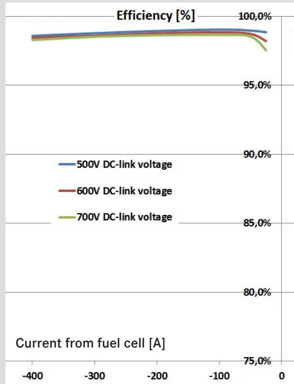
Fig. : Efficiency curves are valid for DCDC200 and DCDC200-HL. Current flows into DC Link
